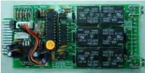
Fig. 8-3-5 - 1 Relay contact card (DCE-B card)
