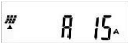
Fig. 7-4 - 8 Display N - String A current
