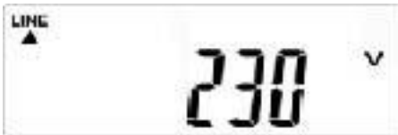
Fig. 7-4 - 12 Display R - Output voltage of the photovoltaic solar inverter
