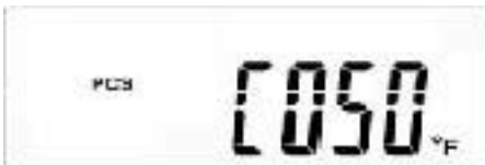
Fig. 7-4 - 4 Display J - Internal temperature of the photovoltaic solar inverter in °F
