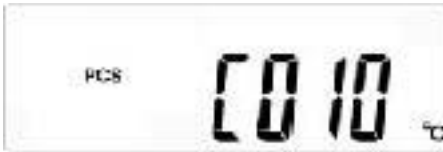
Fig. 7-4 - 2 Display H - Internal temperature of the photovoltaic solar inverter in °C
