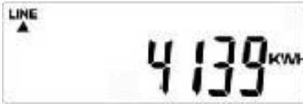
Fig. 7-4 - 1 Display G - Total feed power
